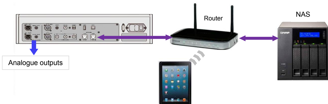
Figure 2 – Using a Rossini DAC with a NAS
