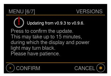
Please note: depending on the type of update the install can take up to about 15 minutes. During this time you will not see information on the display, the power LED fading quickly and the power button on the back is disabled. **Please remain patient and do not unplug the device while updating** since this will cause the update process to fail and the procedure starts again when the device is powered up.
