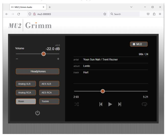
There are two sections: on the left is the control area. You can change the volume and select a source. Below the inputs you can find the stand-by button.
