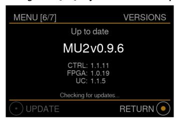
In this menu you can view the current software version and start an update. The MU2 automatically checks for an update every hour and also when entering this menu page from menu page [5/7]. If the MU2 is checking for updates, this is shown at the bottom of this menu.
