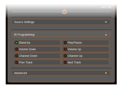
The infrared remote functionality requires an IR extension cord connected to the 3.5mm jack on the back. Please see the hardware manual for the connector location and pinout information.
