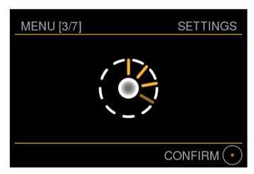
Turn the main knob clockwise to increase the brightness and counter-clockwise to decrease the brightness. Please note that the LED can not be turned off completely to facilitate showing whether the MU2 is in operation/stand-by or power off.
