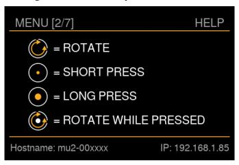
This menu shows the pictograms that are used in the MU2 for operating the main knob. At the bottom of the screen the current network information is shown. The indicated hostname depends on the serial number of your MU2. If the IP address shows 'unknown', there is no network connection and in that case the MU2 cannot be found by the Roon App in your tablet or smart phone. In that case, please check the network connection of your MU2.
