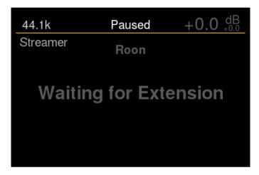
If Roon is running but there is no Roon remote (such as your iPad) connected yet, the message changes to "Extension Connected". If a Roon remote is present, the latest track info is displayed (see below). If none of these happen, the Extension is not activated, Please read the chapter Extension to enable track information on the MU2 display.
