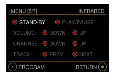
The dot will turn orange until the MU2 receives an infrared command. Press the desired button on your infrared remote to link this infrared command to the selected function. When the MU2 receives an infrared command the dot will turn green and it returns to the infrared selection menu as shown in the previous image.
