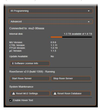
In case your MU2 has an internal Music disk, its free space and the total space of the disk are shown. Note that the displayed disk space will be somewhat lower than advertised as this is in "JEDEC 100B.01" format which differs from the "IDEMA" standard used by disk manufacturers.
