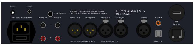
The MU2 is shipped with a proper mains power cable, use this to connect the MU2 to a mains outlet<sup>1</sup>. The MU2 works with nominal mains voltages from 100V to 240V.
