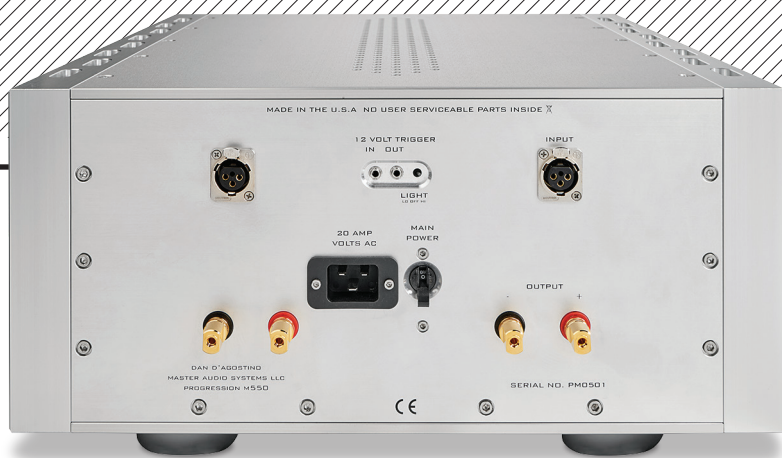
ABOVE: A pair of balanced XLR inputs are paired with gold-plated 4mm speaker cable binding posts. There's a power breaker next door to the flat-blade IEC mains inlet while, above, a tiny three-position toggle sets the meter's green illumination
